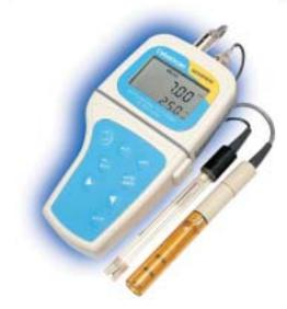
Eutech's multiparameter Waterproof CyberScan PC 300 meter is IP 67 rated and packed with advanced features. Meter is designed to use separate probes for pH and Conductivity.
