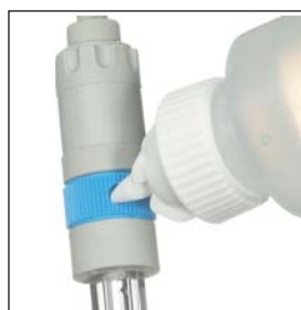
Pour in reference electrolyte with the refilling bottle (that is supplied with all electrodes)
