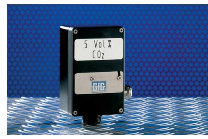
Transmitter with infrared (NDIR) sensor One-man calibration on-site Output 0.2 .. 1 mA or 4 .. 20 mA Long lifetime, low maintenance cost
