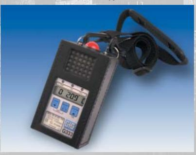
high-quality electrochemical sensor and gives alarm for both oxygen deficiency <u>and</u> oxygen surplus.
