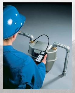
helix-cable allows to carry the G300 II in the pocket to watch out for leakages with only the sensor in one hand. A combination of gooseneck and helixcable gives you access to far away spots. Both the sensor and the extensions can be mounted without tools.
