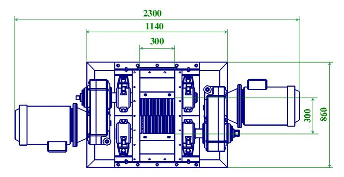
**Drive:** 2 Geared motors. Voltage: 2 X 400 V, 50 Hz.
