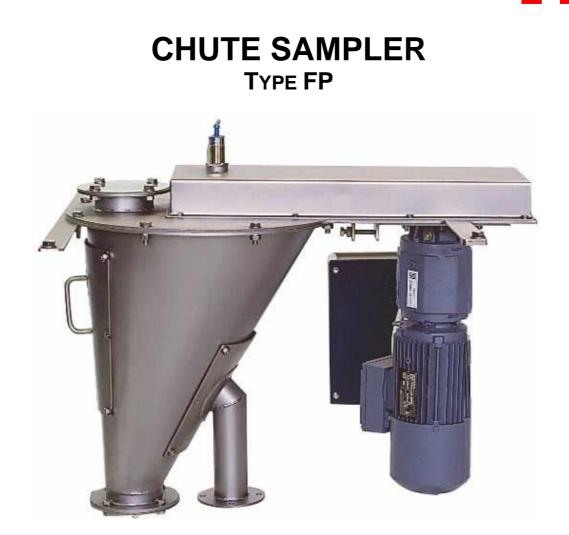
The **Chute Sampler Type FP** is designed to take out increments of none-sticky powdered material and lumps up to 40 mm, in a closed pipe system, from a free falling flow of materials.
