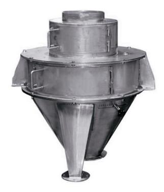
The **Disc Divider** is used for dividing samples of powder and bulk materials (even suitable for wet materials). The main advantage of mechanical sample dividers is that they extract a part of the material by a large number of increments. If less than about 50 increments are taken by the sample divider, the accuracy may be substantially reduced. A continuous automatic sample division ensures that the divided sample is still a representative sample.
